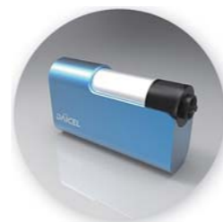
A prototype drug administration device, developed as part of basic research, employs explosives engineering technologies to deliver medications into living tissues
