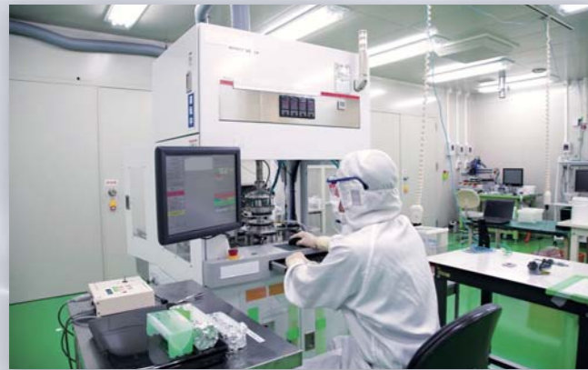
Wafer level lens production facilities are isolated in a clean room to thoroughly minimize the possibility of contamination by foreign matter.
